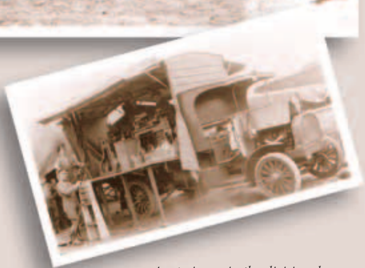
A repair car in the divisional ammunition park. Notice the chain-operated transmission and solid-tired wheels. [LAC PA 16]
