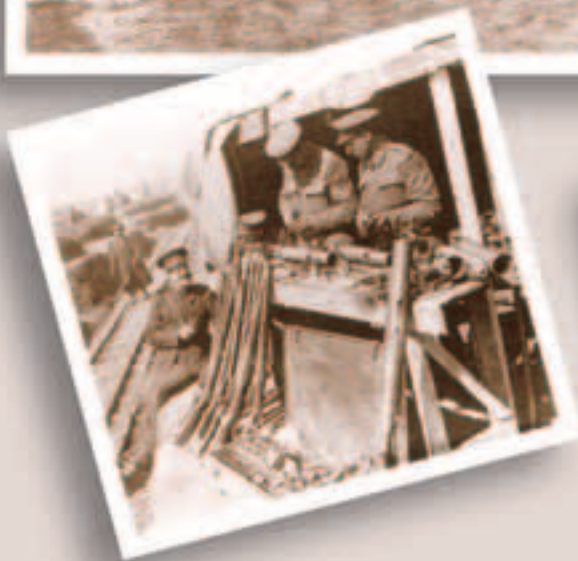
Armourers repairing rifles and machine-guns in a mobile workshop conveniently situated beside the light railway leading to the front. [LAC PA 1272]
